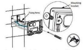
Make sure the cistern is fully commissioned before mounting the bracket in place. Locate the mounting bracket onto the fixing arms and secure the top left and bottom right corners with the screws provided and tighten with a screwdriver. Be careful not to overtighten. Re-connect the clip links and cable ribbon to the glass cover and insert the battery holder. Reinstall the glass plate. Once correctly installed the flush plate will illuminate for a couple of seconds.
