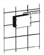
After you have chosen the ideal location for your sensor flush plate. Use the control panel base to mark where you wish to install the flush plate.
