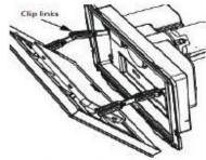
Remove the glass panel completely. Push the glass front down from to the top and tilt the top towards you. Un-clip the glass by expanding the clip links and keep aside until installation is completed.
