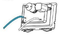
Connect the air hoses from the cistern to the flush plate as shown. Attach the blue hose to the semi-circle symbol and the transparent hose to the full circle symbol.
